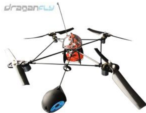
FIGURE 3 – DRAGANFLYER SAVS STABILIZED AERIAL VIDEO SYSTEM GYRO STABILIZED RC HELICOPTER (DRAGANFLY INNOVATIONS INC., 2007)
